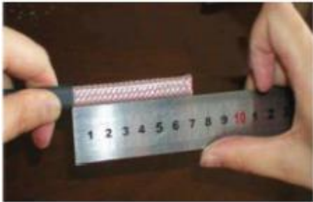
Figure 3 3. Lightly score completely around and then down inner jacket. The length is 45mm (1-4/5").
