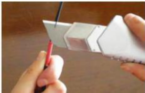
Figure 7 7. Cut center matrix away, leaving bare conductors. Do not cut bus wires!
