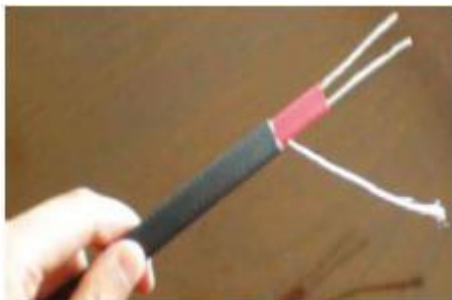
Figure 9 8. Slide 3.2mm (1/8") x 25mm (1") shrink tubes over bus wires. To shrink tubing move heat source continuously from
