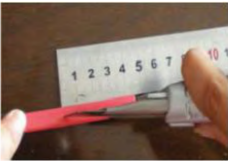
Figure 5 5. Skive outer matrix material from conductors with utility knife.
