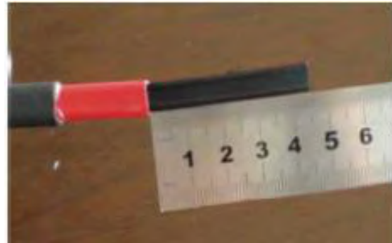
Figure 6 6. Peel exposed wires back from center matrix.
