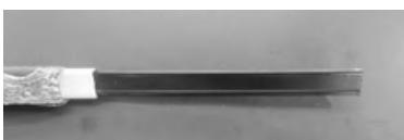
12. Pull back bus wires then, carefully strip bus wires.
