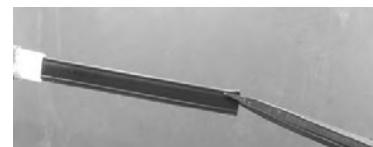
13. Carefully cut the center area (core) between the two bus wires.
